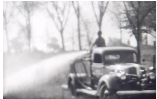
1940 Ford Pumper with a rolling pump and 800 gallons of water.
