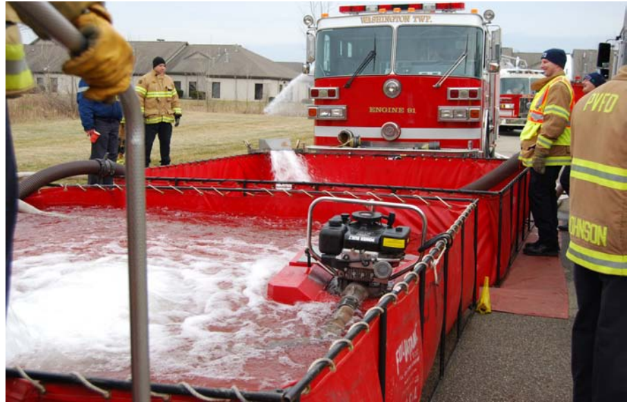
Pleasant Valley, Liberty and Jerome Township Fire Departments helped Washington Township test the Fire Department's ability to supply non-hydranted water at a rate of at least 400 gallons/minute for two hours to a scene. This tanker operation is a requirement of the Insurance Service Office for a Class 1 rating.
