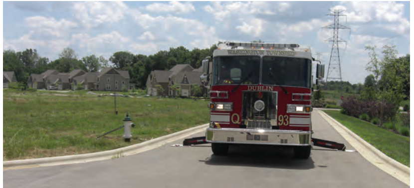
Quint 93 is parked on Winemack Lane in the Tartan development. Stabilizing outriggers which are extended when the 75-foot ladder is in use, increase the space needed for the vehicle.
